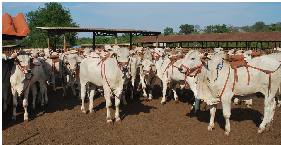
Fig 1. Animals, in a test group, with the apparatus (halter, saddle and cylinder) for methane collection by sulfur hexafluoride ( \text{SF}_6 ) tracer gas technique.
