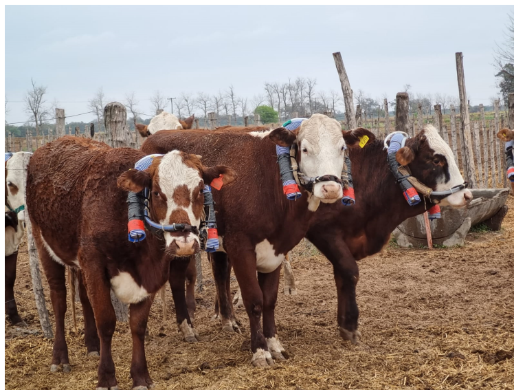
Figure 1. Experimental animals equipped with devices for measuring enteric CH 4 emissions using the SF 6 tracer technique. Each animal is fitted with two sample collection systems, housed within a blue corrugated tube designed to contain the equipment. The tube is securely attached to the muzzle.
